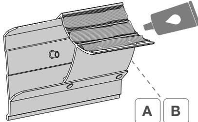
**EN** **Important:** use of SIKA 252 adhesive is essential for fixing the bracket (brackets).
