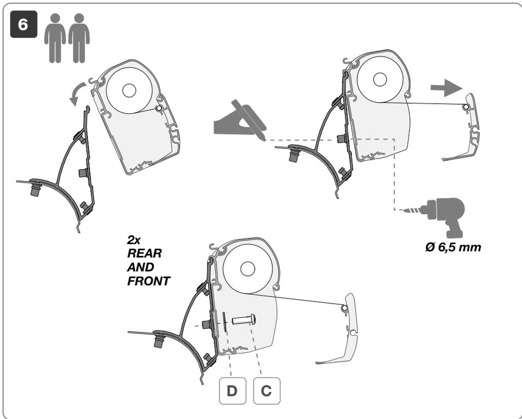
**EN** Before tightening the screws, make sure that the awning position doesn't prevent the opening of the rear door.
